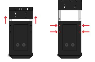
12. Take one **Speaker Bar** and attach the **2 cables** to the top half of the Main Unit, then secure the speaker bar using **4 Phillips screws**.
