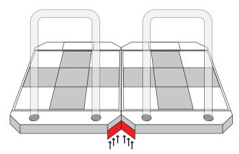
7. Install the second **V-bracket** to the **front** of the stages in the same way the rear V-bracket is attached with the silver-side upwards. Use **6 M8 screws, lock washers, and washer** to secure.
