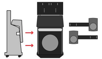
11. Raise the **monitor mount** by sliding the top half of the main unit upwards.
