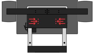
14. Connect the AC power cable to the back of the Monitor, making sure the red latch has locked.
