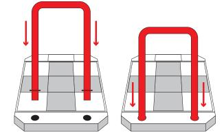
3. Securely tighten both bolts into the support bar from **underneath** the stage using a wrench.
