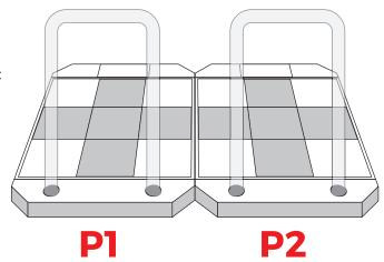
Using one of the included V-brackets and 6 included M8 screws, lock washers, and washers, attach the bracket onto the back of the stages.
