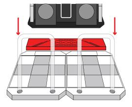
Connect BOTH of the USB-C Data Cables and 12V DC Barrel Plugs from the Stage Connector Platform to each stage.
