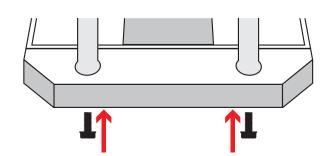
4. **Stabilize** the stages from movement and vibrations by loosening the wingscrew and spinning the red tightener on each stage's wheels counterclockwise until the stage is raised off of the wheels and leveled.
