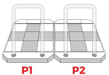
Using one of the included V-brackets and 6 included M8 screws, lock washers, and washers, attach the bracket onto the back of the stages.
