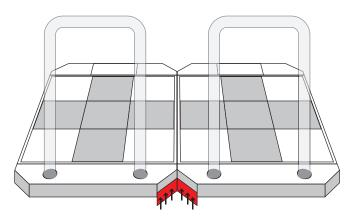
Install the Triangular Cover bracket to the front of the stages in the same way the rear V-bracket is attached with the silver-side upwards. Use 4 M8 screws, lock washers, and washers to secure.
